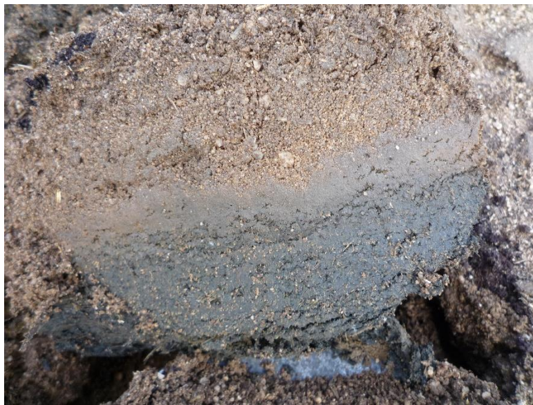
Figure 3. Soil textural layers are impervious to water movement and can become anaerobic, as indicated by the blue-gray color (reduced form of soil metals under low oxygen conditions). Photo by Jim Downer.
